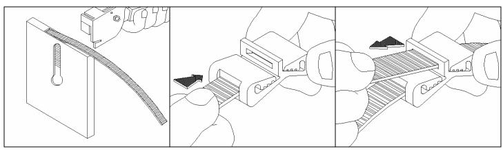
1. Cut Q-Band to length, allow 2-3 inches of excess material for tool to grip the band.
